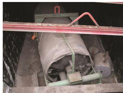
Stored RAW – VVR-S research reactor vessel
