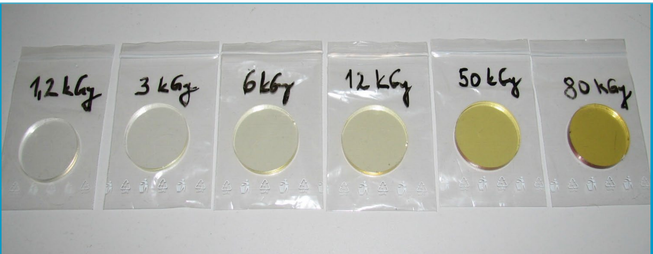
Radiation induced colour change of plexiglass – testing the radiation resistance of camera system and lights for reactor pressure vessel inspections
