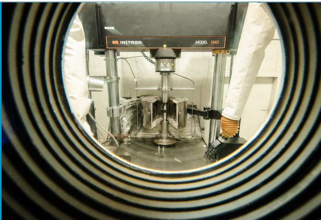
Static fracture toughness testing of irradiated materials (using 0,5T-CT specimens)
