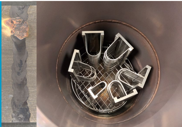
Autoclave vessel with different sets of metal samples
