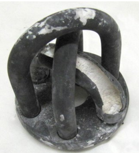
Destruction of a heating element
