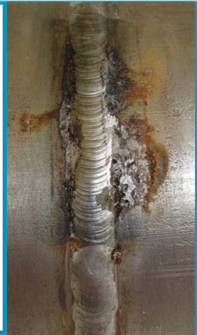
Microbiologically induced corrosion the piping from the austenitic stainless steel – SEM micrograph (left) and the defect on the outer surface (right)
