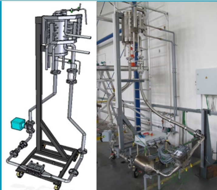
BESTH-2: Small scale Experimental Facility for IVMR experiments
