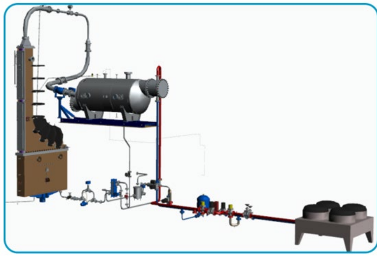
THS-15: Large scale experimental facility for IVMR experiments
