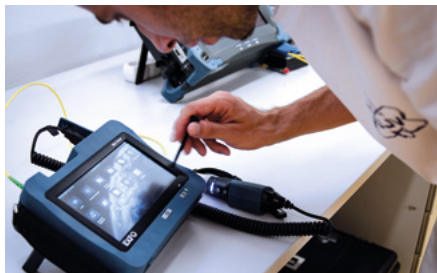
Fiber optic cable qualification; attenuation measurement with LSPD (Light Source and Power Meter) devices and/or OTDR (Optical Time Domain Reflectometer).
