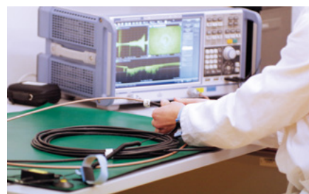
Vector network analyser (VNA) for monitoring of high frequency changes of communication cables and HF equipment.
