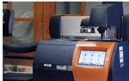
Differential scanning calorimetry (DSC) for thermal properties measurement.
