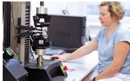
Determination of tensile properties of polymeric materials.
