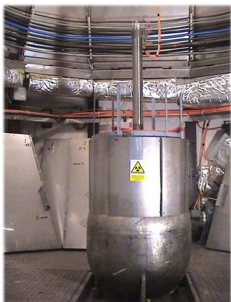
Container with the cobalt source in the standby position.
