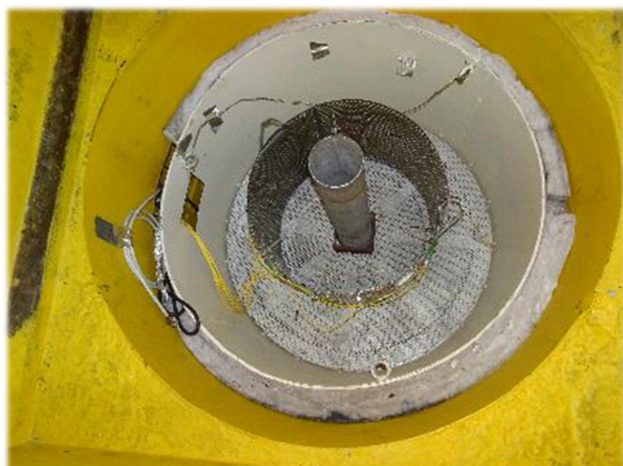
Fiber optic components inside the box at room temperature with functional measurement.
