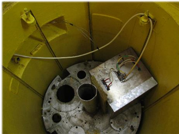
Box for irradiation at 300 °C.
