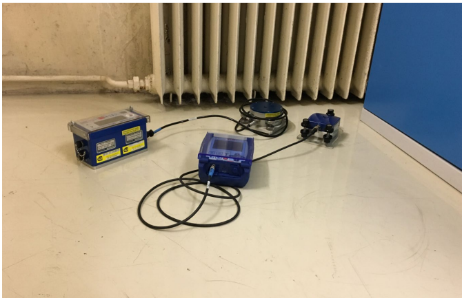
Seismograph placed in the basement of the LVR-15 building to measure the response from the Klecany quarry blasts
