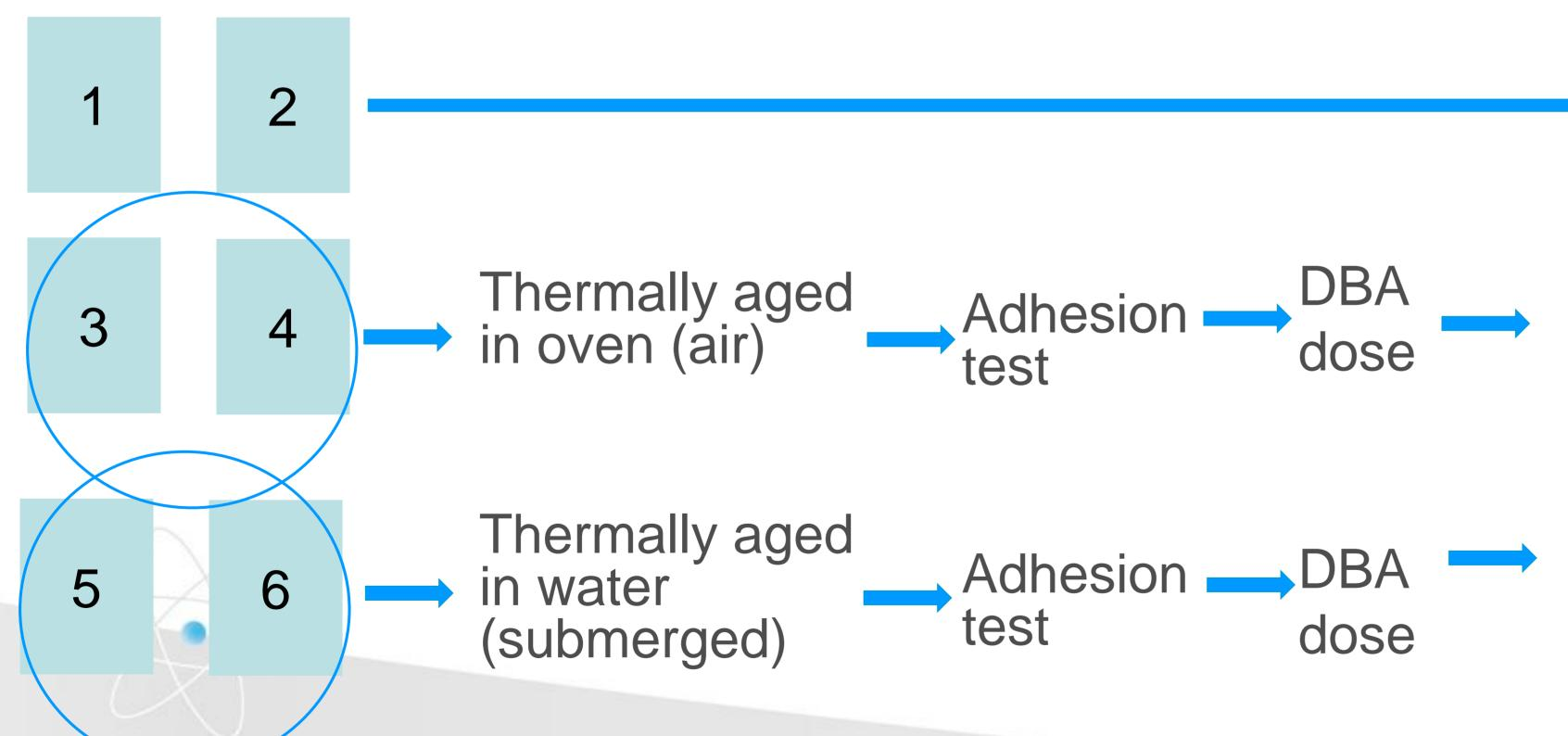
Test coatings with applicable t-T-P curves simulating DBA atmosphere
