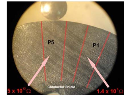
$IR = 1.0 \times 10^9 \Omega = 12 \text{ M } \Omega \cdot 1000 \text{ ft}$
