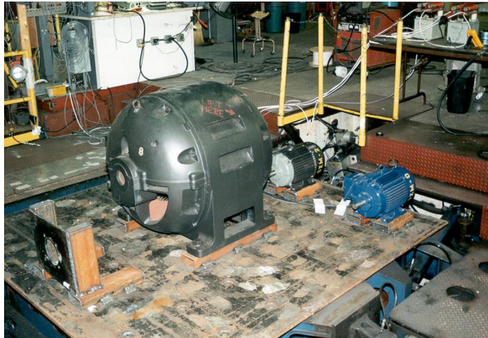
Random and Form Wound Motor Specimen Undergoing Seismic Test Courtesy: Schulz Electric
