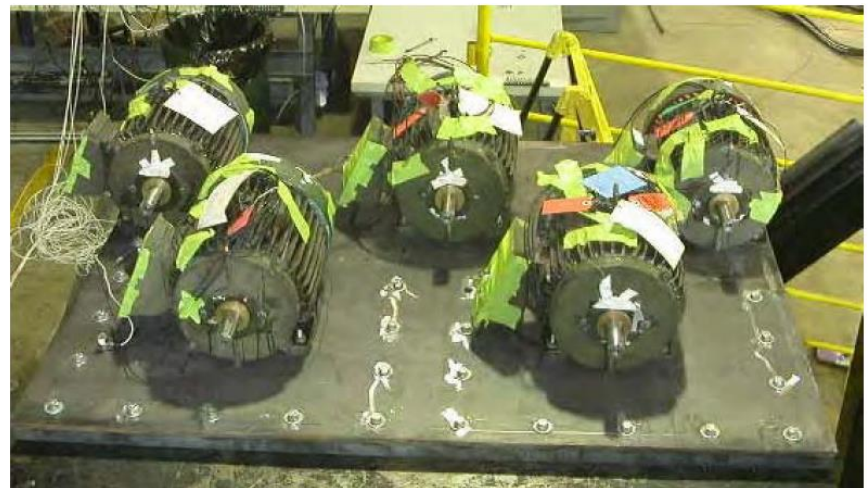
Random and Form Wound Motor Specimen Undergoing Vibration Aging - Courtesy: Schulz Electric and EPRI
