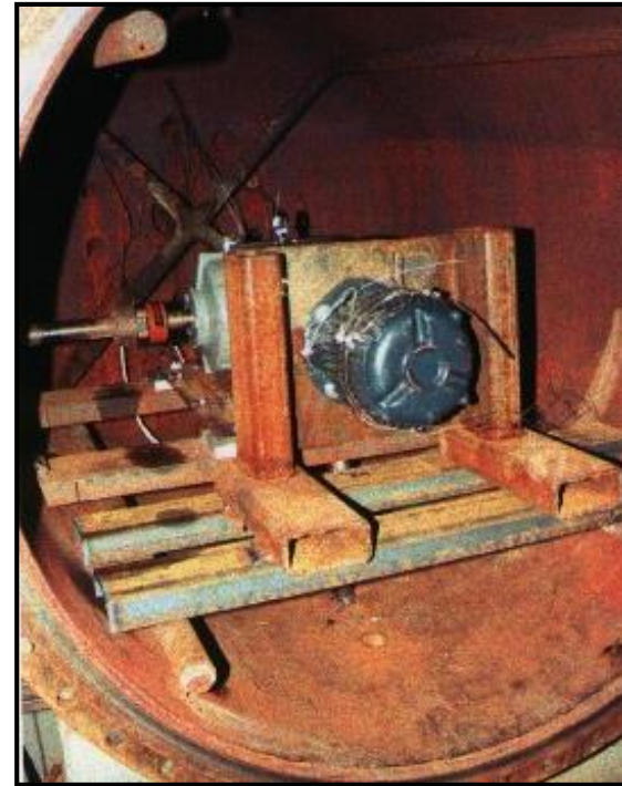
MOV Motor Specimen inside LOCA Chamber Prior to MSLB/HELB
