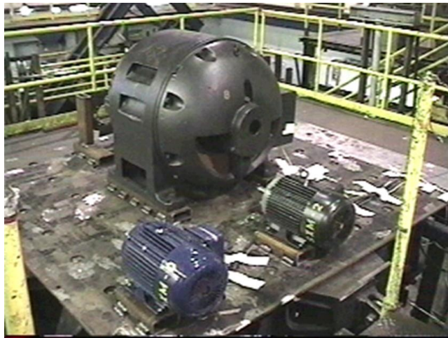
Random and Form Wound Motor Specimen Undergoing Vibration Aging - Courtesy: Schulz Electric and EPRI
