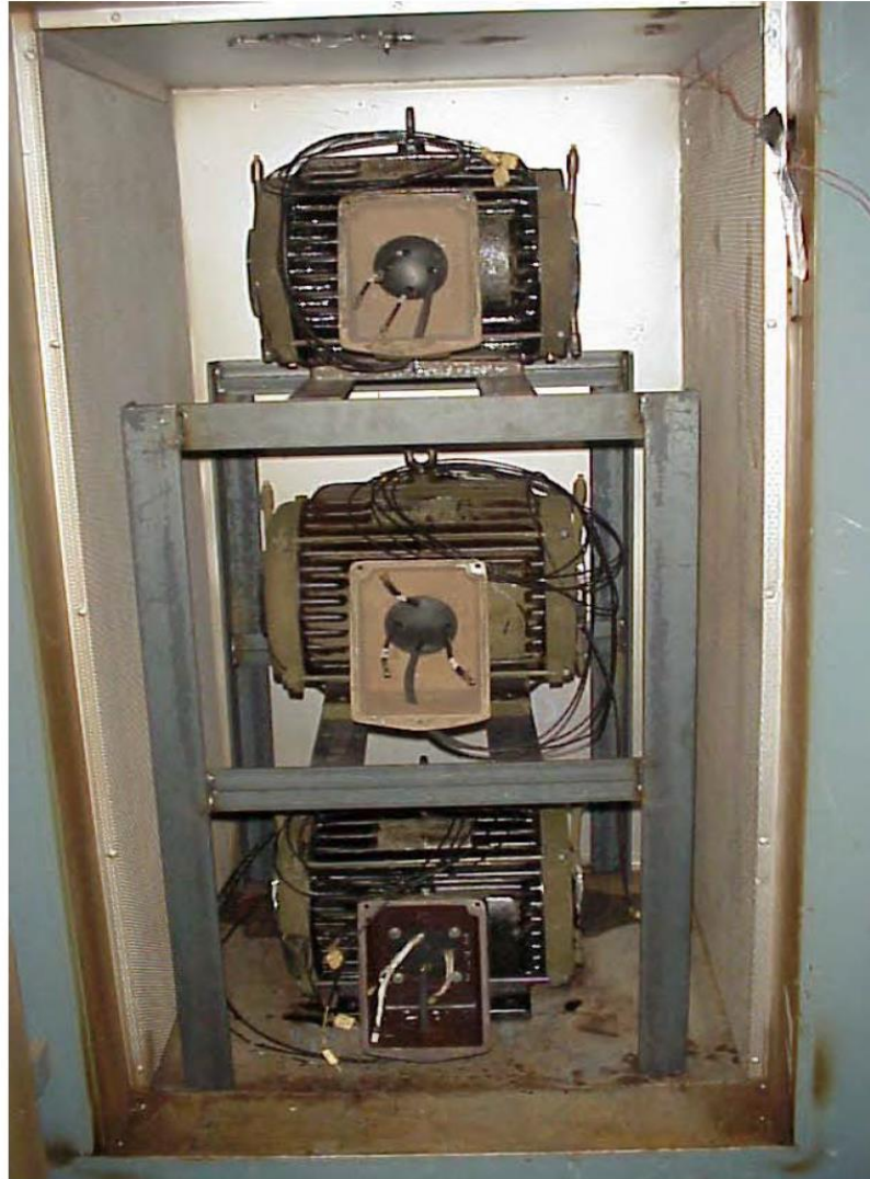
Random Wound Motor Specimen Undergoing Thermal Aging Courtesy: EPRI
